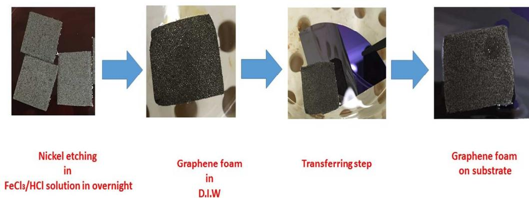
**Figure S1.** Transfer of graphene foam on substrates.
