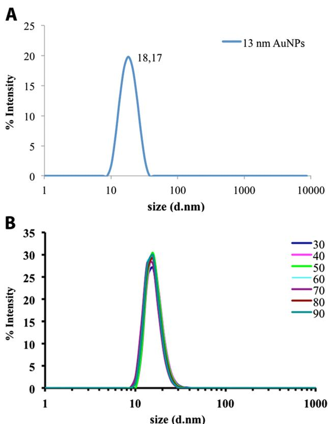
Figure 2. Hydrodynamic radii image of 13-nm AuNPs (A). Dynamic light scattering spectrum of 13-nm AuNPs (B).
