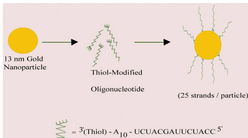
Figure 1. Schematic representation of 13-nm AuNPs modified with thiolated oligonucleotides.
