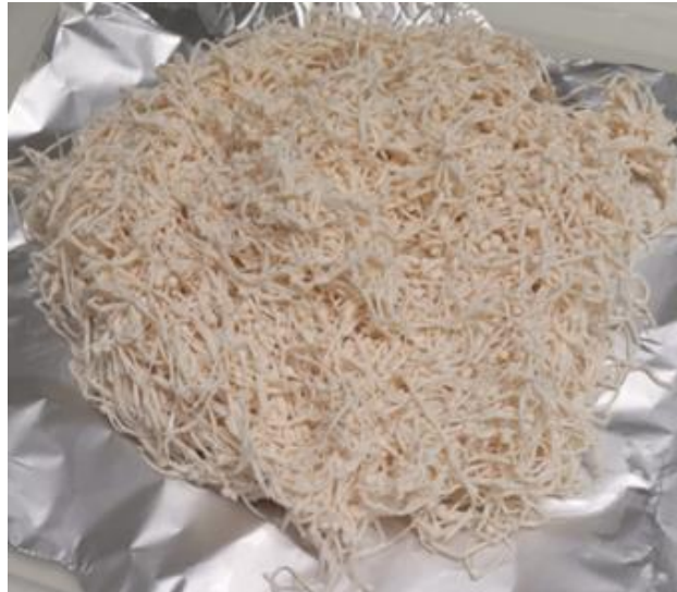
Precipitated SPEEK polymers
